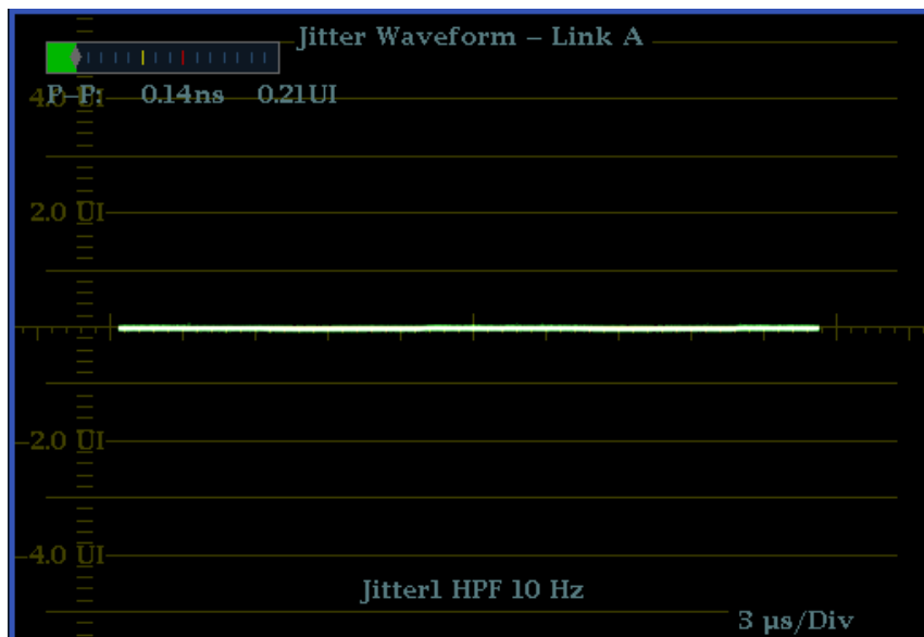
Figure 30: The Jitter display parameters as shown in a single tile when the instrument is in 4-tile mode
